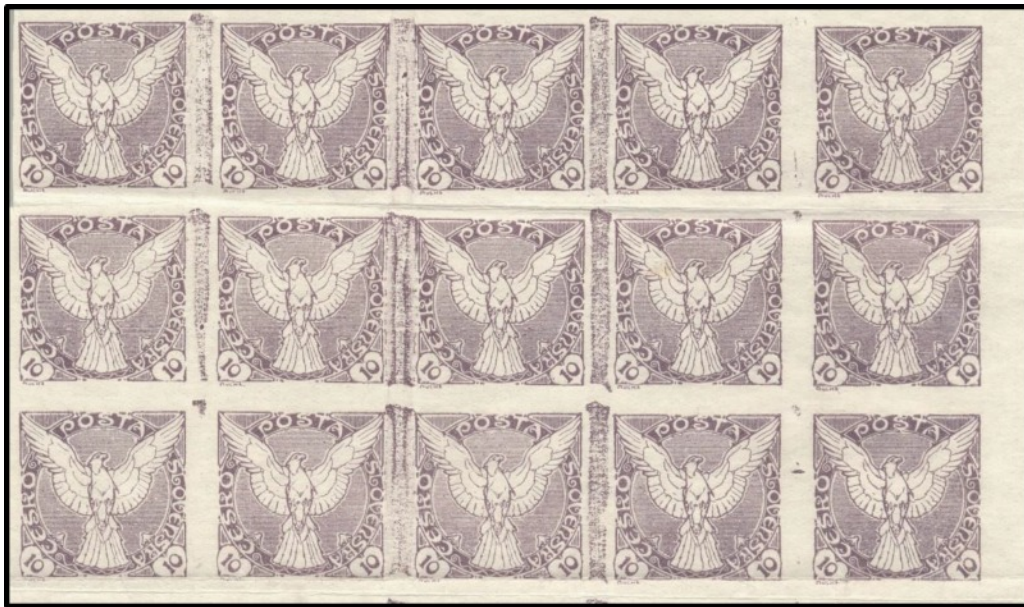
Fig. 1: Plate 2. An air cushion under the sheet when it was placed on the press caused the paper to receive ink between the clichés.
